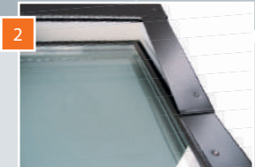
UV resistant cladding made from coated aluminum for long-term performance. Aluminum covering the entire sash's boarder to improve the window's performance. Aluminum's back side covered with a particular plastic to avoid condensation effects.
